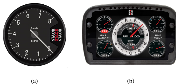
Fig. 1. (a) Analog needle gauge [33] and; (b) skeuomorphic digital display emulating analog gauges [32].
