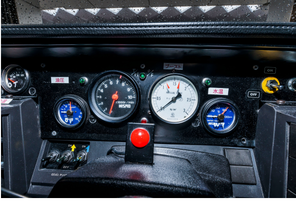
Fig. 2. Analog gauges fitted to 1987 Nissan Skyline GTS-R Group A race car [2].
